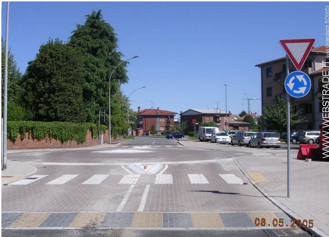
Figure 2 - Mini-roundabout with raised kerb
